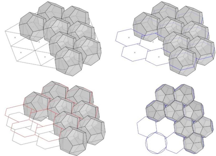
Fig. 2: Topological interlocking of pentagonal dodecahedra.
