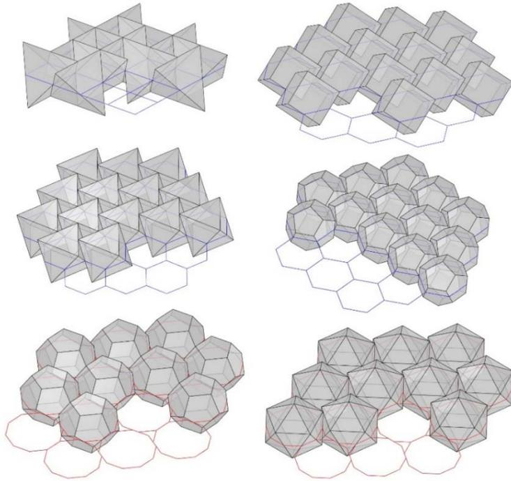
Fig. 1: Topological interlocking of convex regular polyhedra.
